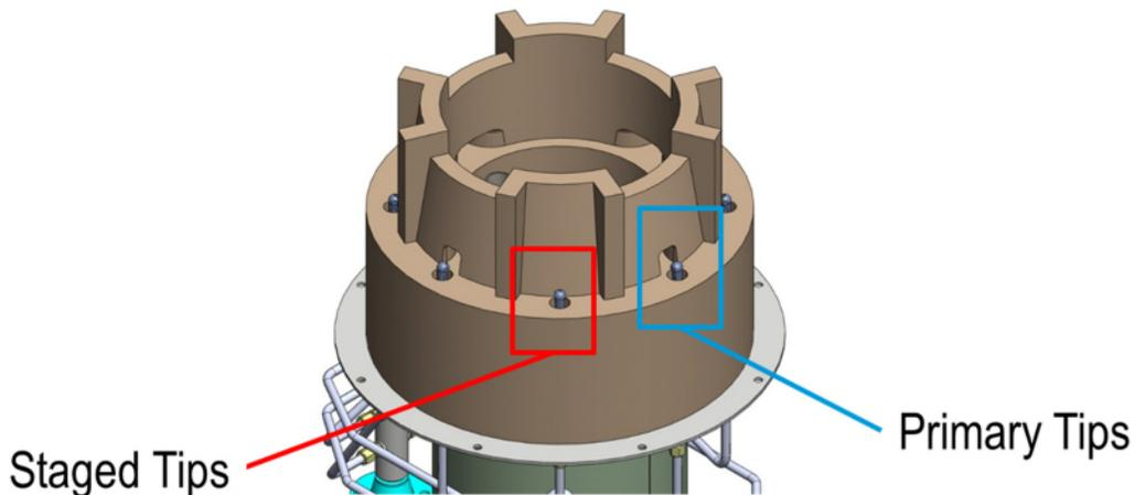
Figure 12 Advanced burner tile design to help minimize NO<sub>x</sub> formation.
