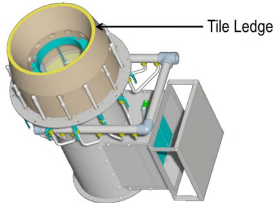
Figure 4 Burner tile with a ledge at the outlet.
