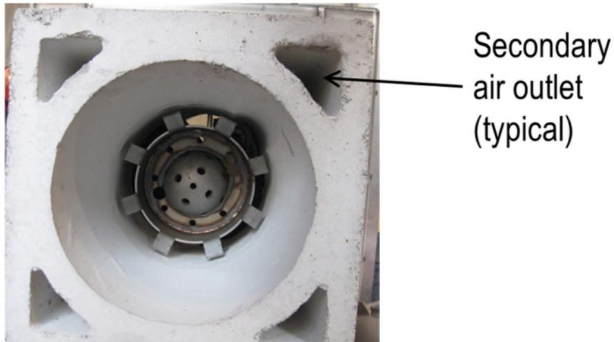
Figure 6 Burner tile with 4 secondary air outlets.
