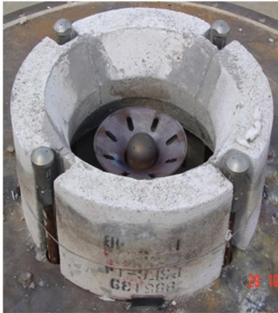
Figure 14 New burner tile with four segments.
