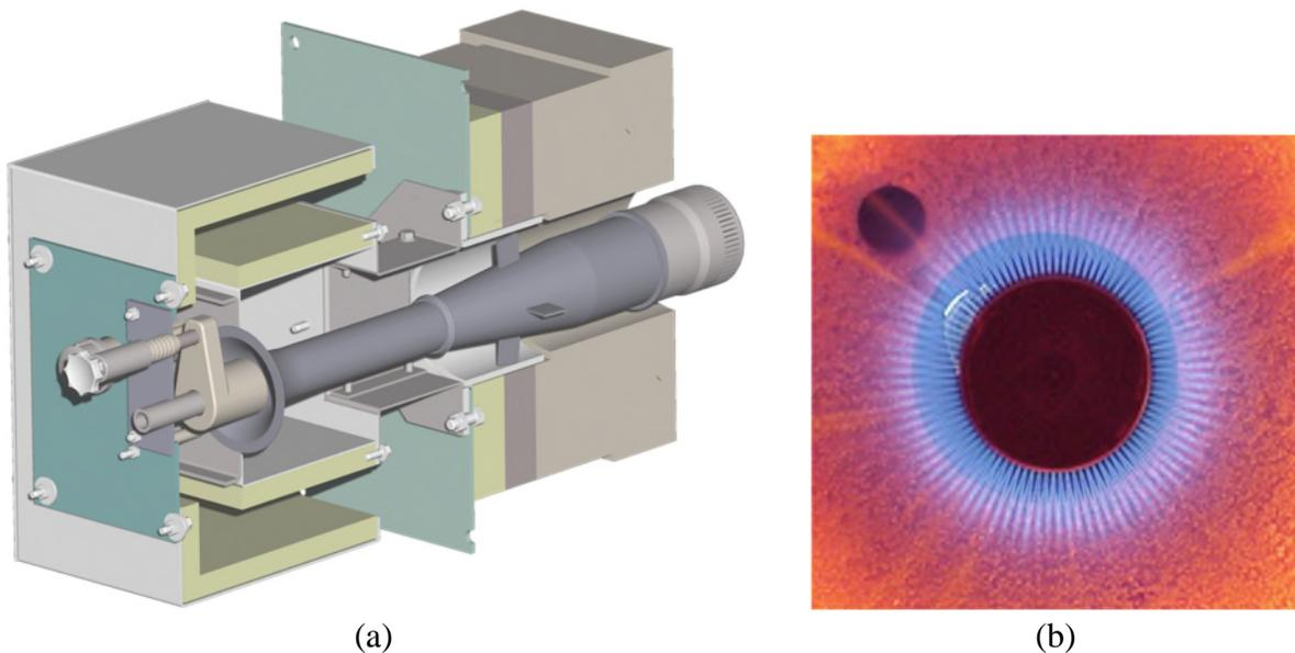
Figure 1 Radiant wall burner: (a) cutaway, (b) photo of burner radiating in a furnace.
