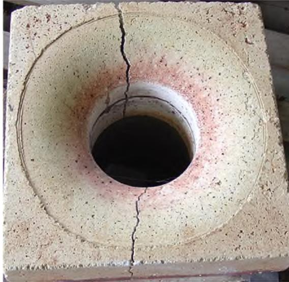
Figure 17 Cracked burner tile.
