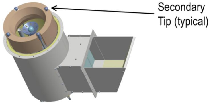
Figure 11 Burner tile with secondary fuel tips in the tile.
