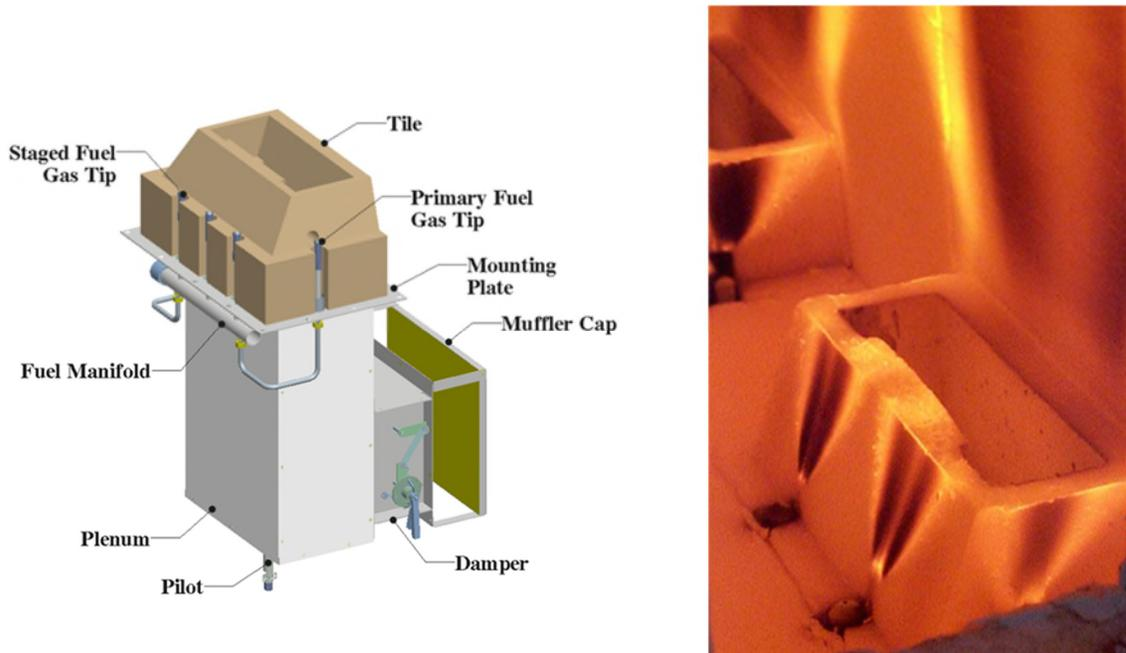
Figure 10 Burner with a rectangular tile.
